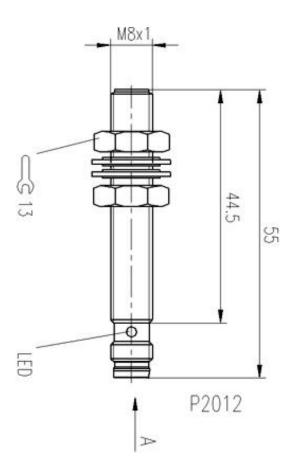
**Inductive Sensors** BES 516-324-G-S 4-C M8x1 x 70,5 normally-open Sn=2mm shielded
